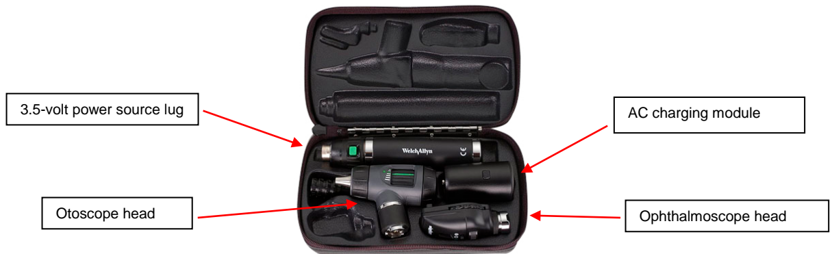
Figure 5: Otoscope and Ophthalmoscopes Parts
