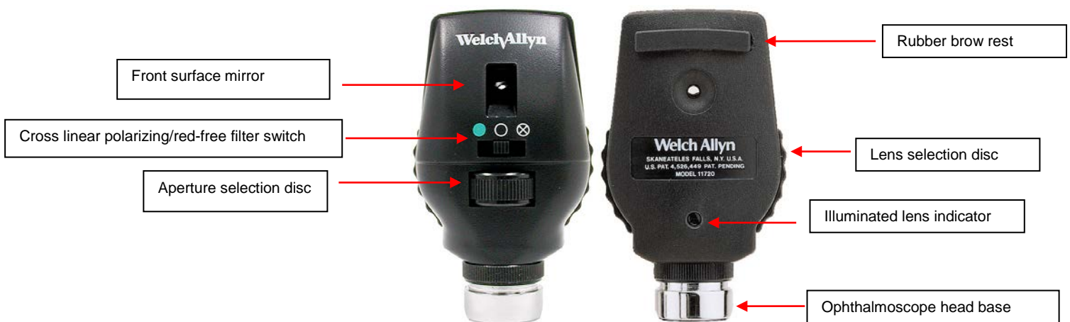
Figure 3: Using the Ophthalmoscope
