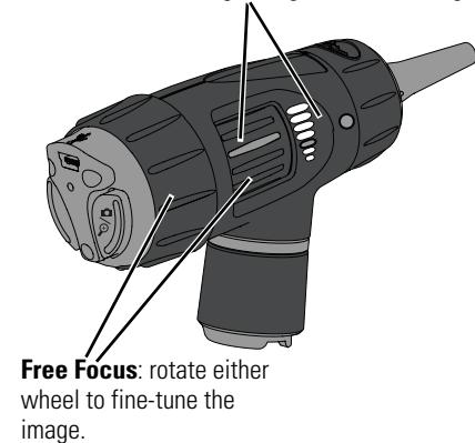
**Free Focus:** rotate either wheel to fine-tune the image.
