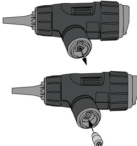
It is necessary to re-calibrate the white balance on the Digital MacroView after replacing the lamp.
