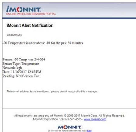
**Figure 1: Email notification of temperature excursion based on the setup parameters for each sensor.**
