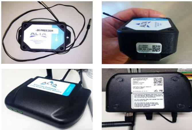
Figure 9: iMonnit wireless temperature sensor monitor, gateway, and identification stickers.
